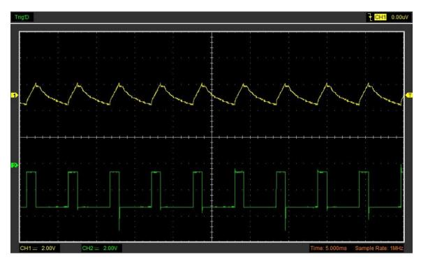
The longer pulse width (channel 1 output of the emitter, channel 2 driver pulse from Pire Plus Eval Board) Note: that the intensity is higher but its percent modulation depth is less.
